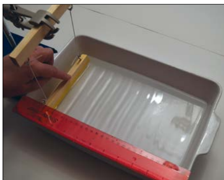
This cheap and controllable ripple tank is made from a lasagne dish.
