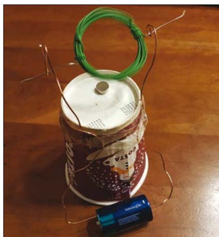
A motor built from bits and pieces found lying around in "Mentors, motors and merch" (podcast 9).
