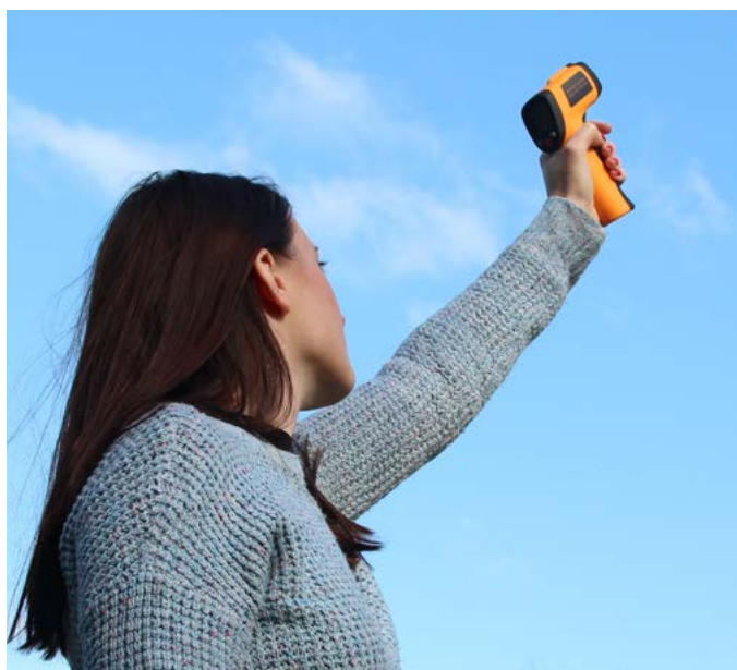
Figure 1: Measuring the temperature of the sky with an infrared thermometer
