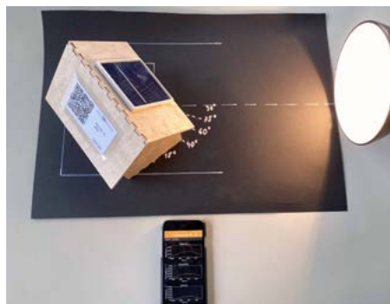
An experiment to explore the angular dependence of a solar cell's power output.
