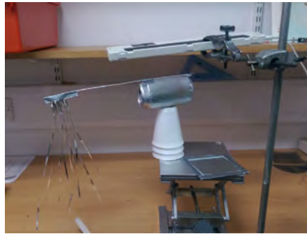
Demonstrating the photoelectric effect with an aluminium can and polystyrene cups
