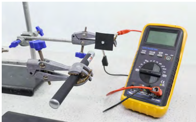
Equipment set up for LED photocell activity
