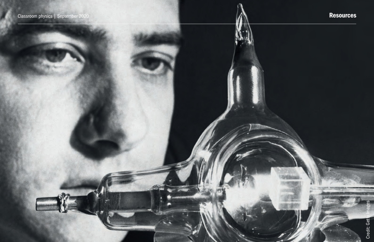
Dr. Theodore H. Maiman, of Hughes Research Laboratories studies a ruby crystal in the shape of a cube in a laser (Light Amplification by Stimulated Emission of Radiation) which is the essential element in a new electronic device. Date taken: 07 July, 1960
