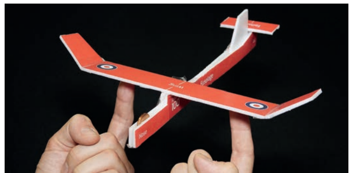
Figure 1. The glider's C_M can be found by finding the point at which it balances. Top: A glider (without a penny) suspended by string at its C_M ; Bottom: A glider (with a penny) balanced on two fingers.
