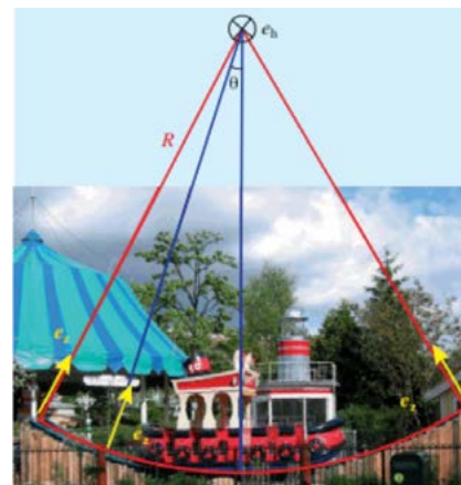
The ride and the radius of the circular arc of the rail, which takes the place of the string in a pendulum
