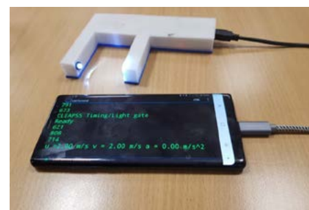
A mobile phone displaying data from the CLEAPSS light gate.
