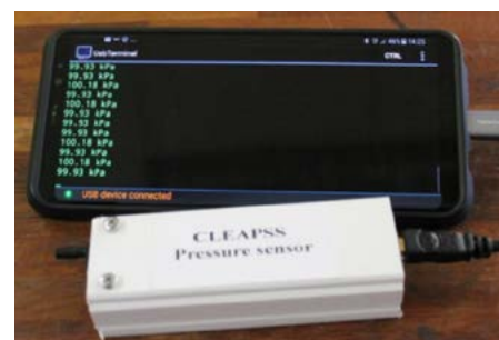
A mobile phone displaying data from the CLEAPSS pressure sensor.
