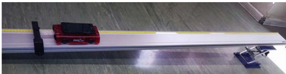
Experimental set-up for the study of acceleration of a smartphone moving on a ramp.
