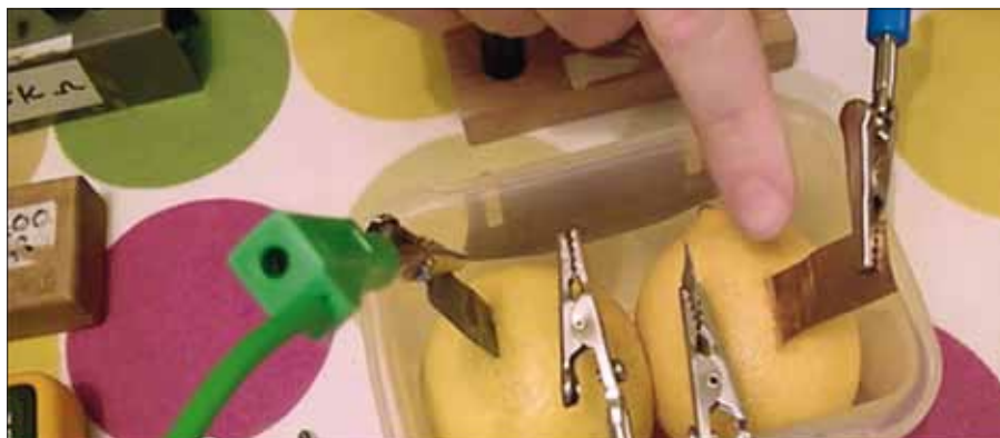
Lemon batteries are used to light an LED, in Dan Cottle's Real Physics with Fruit and Sweets .
