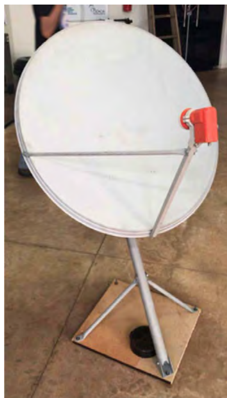
The home-made radio telescope
