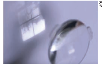
Image of a window focussed onto a sheet of paper using a fat lens (4.5 cm focal length).
