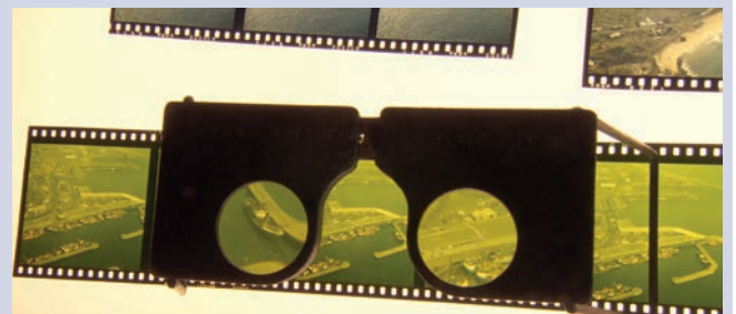
A stereoscopic viewer of the type used for aerial reconnaissance during the Cold War.
