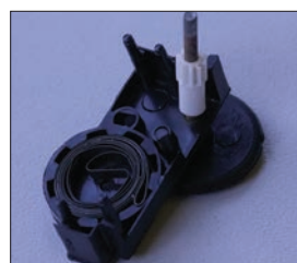
Above: An energy mouse. Left: A dissected mouse showing the coiled spring, which stores energy elastically.
