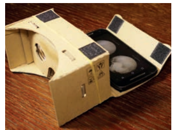
A viewer with a mobile phone and fat (short focal length) lenses mounted.
