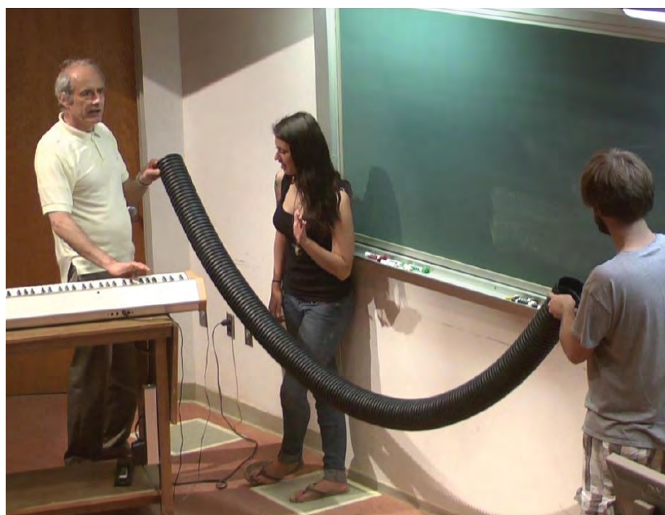
The monster sound pipe: the keyboard is used to match the frequency when the tube is smacked. The matched tone is found to be a semitone lower than the theoretical predicted value.
