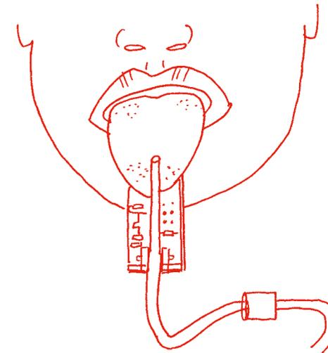
The team has also created a ‘digital lollipop’, a device that can be placed on the tongue to simulate a range of tastes through the application of different currents.
