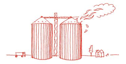
The phenomenon arises because fine powders, such as flour, can acquire a charge as they pass along a pipe. They then discharge to the walls of the silo, causing a spark. A charge as low as  $10^{-3}$  C may be sufficient to create a spark that can transfer 1 mJ. This is enough to have a devastating effect in a highly flammable atmosphere of air rich in flour particles.
