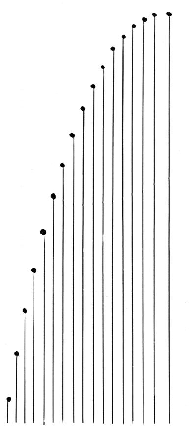
Equal spacing of lines shows a constant horizontal velocity
