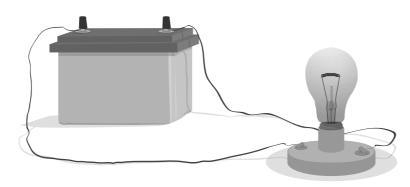
The circuit is left switched on for several minutes. The bulb stays lit all the time. Its brightness does not change.
