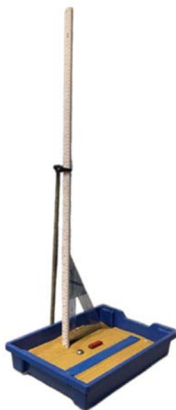
The equipment set up with the ruler clamped into place at the correct angle.
