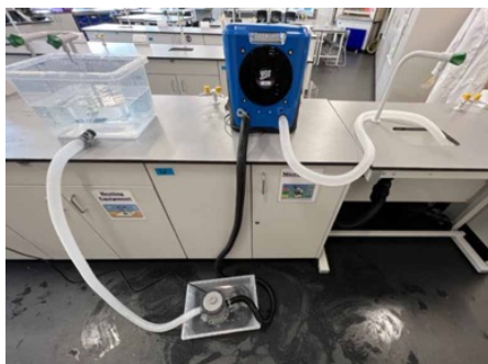
A portable air-source heat pump in the lab.
