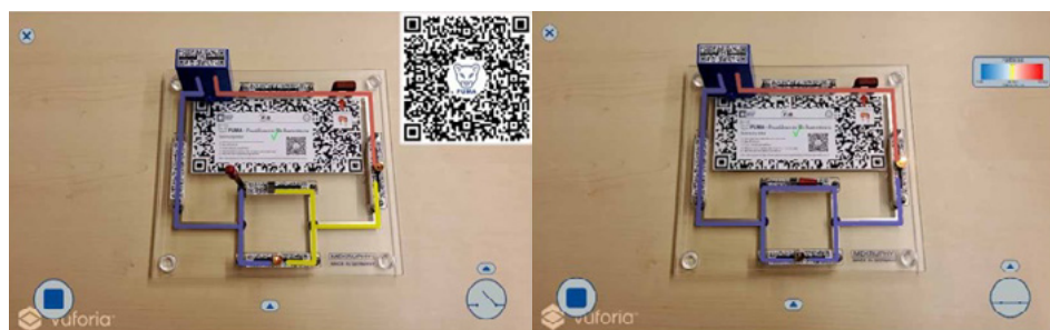
Screenshots from the app showing the effect of closing a switch to bypass a light bulb. Scanning the QR code in the left image prompts a short video about the experiment.
