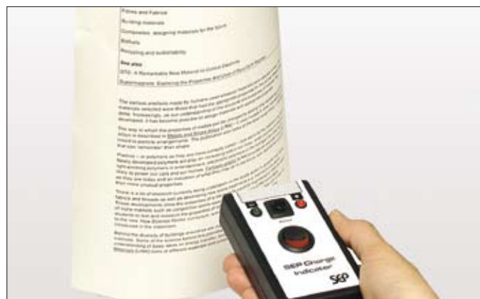
A sheet of paper that has become positively charged on passing through a laser printer loses its charge when it is touched.
