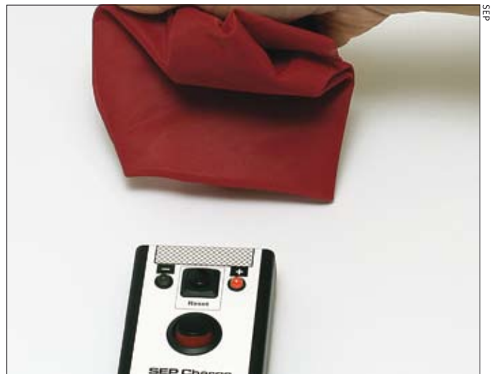
When a polythene rod is rubbed with a nylon cloth the objects acquire opposite charges, as indicated by the SEP Charge Indicator's LEDs.
