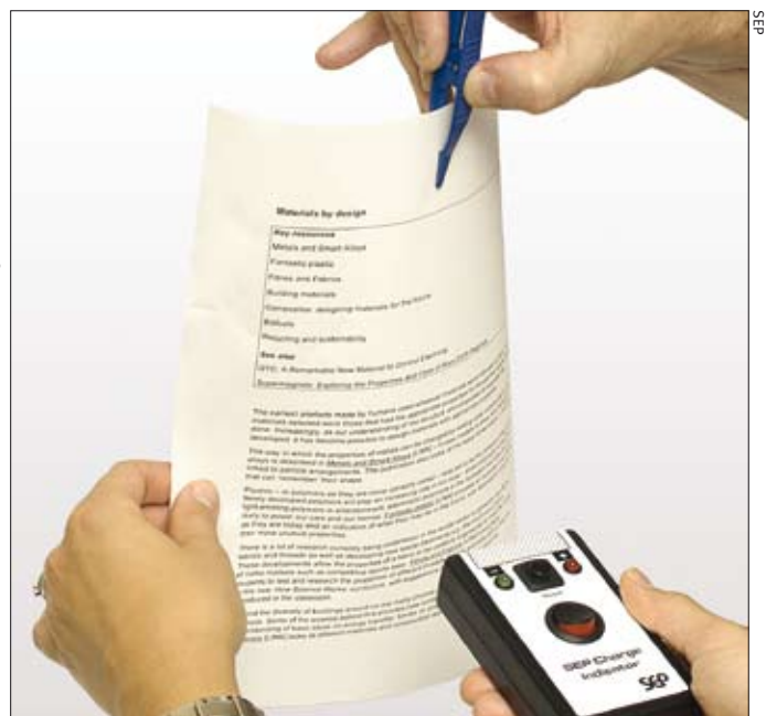
A sheet of paper that has become positively charged on passing through a laser printer loses its charge when it is touched.
