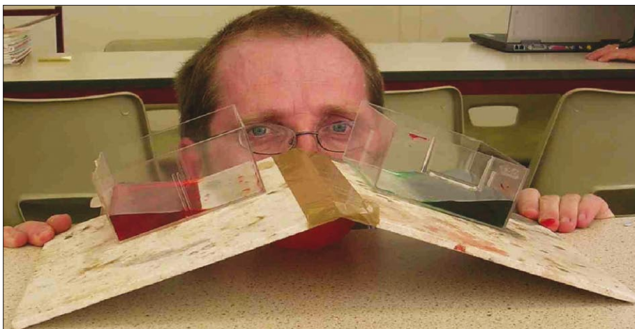
When will it blow? You can predict eruptions by making a tiltmeter in class using minimal resources.
