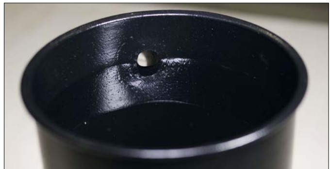
Figure 1 (above): Fill the Eureka can up to the spout hole. Use the measuring cylinder to capture any overflow and then empty the cylinder. Figure 2 (left): Lower the object into the Eureka can. Read off the measuring cylinder the amount of water displaced by the object and hence its volume (1 ml is equal to 1 cm 3 ). Figure 3 (below): An orange with peel is less dense than water. But removing the skin makes it sink.
