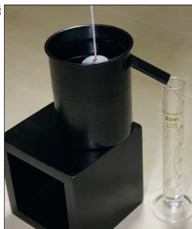
Figure 1 (above): Fill the Eureka can up to the spout hole. Use the measuring cylinder to capture any overflow and then empty the cylinder. Figure 2 (left): Lower the object into the Eureka can. Read off the measuring cylinder the amount of water displaced by the object and hence its volume (1 ml is equal to 1 cm 3 ). Figure 3 (below): An orange with peel is less dense than water. But removing the skin makes it sink.
