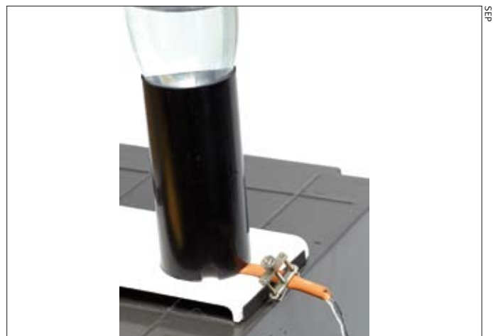
Resting the bottle on the rubber tubing leads to positive feedback.
