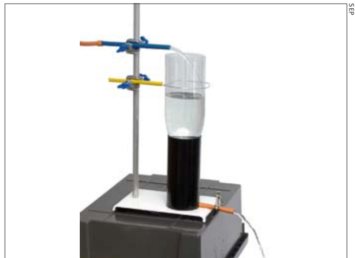
A steady state is achieved when the rates of flow into and out of the bottle become equal.
