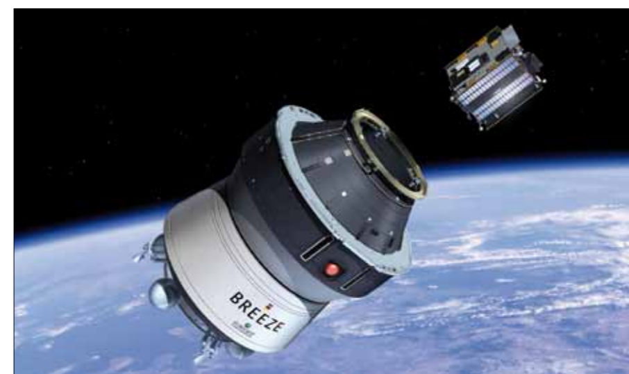
Proba-2 is ejected from the Breeze upper stage of the ROCKOT launcher.
