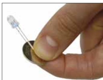
A convenient source of UV radiation is a UV LED and a button cell.
