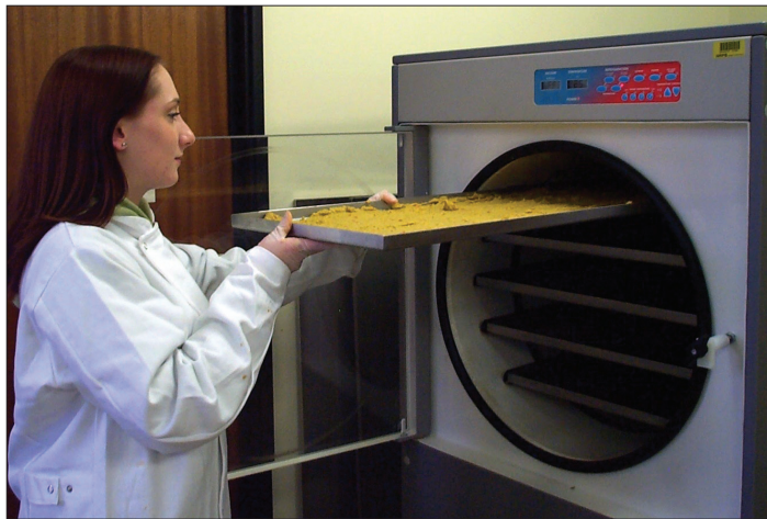
A food sample is dried before radioactive atoms (isotopes) are counted.
