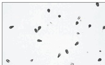
A plastic alpha detector is used to measure levels of radon in a home (left). Alpha tracks in the plastic after the detector has been exposed to gas (right).
